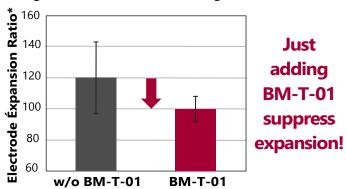
\*Electrode expansion ratio is measured thickness of anode electrode at discharge state (average of 15 cells). The value is calculated by below formula and standardized with BM-T-01 = 100. Error bars indicate 1  $\sigma$  deviation.
